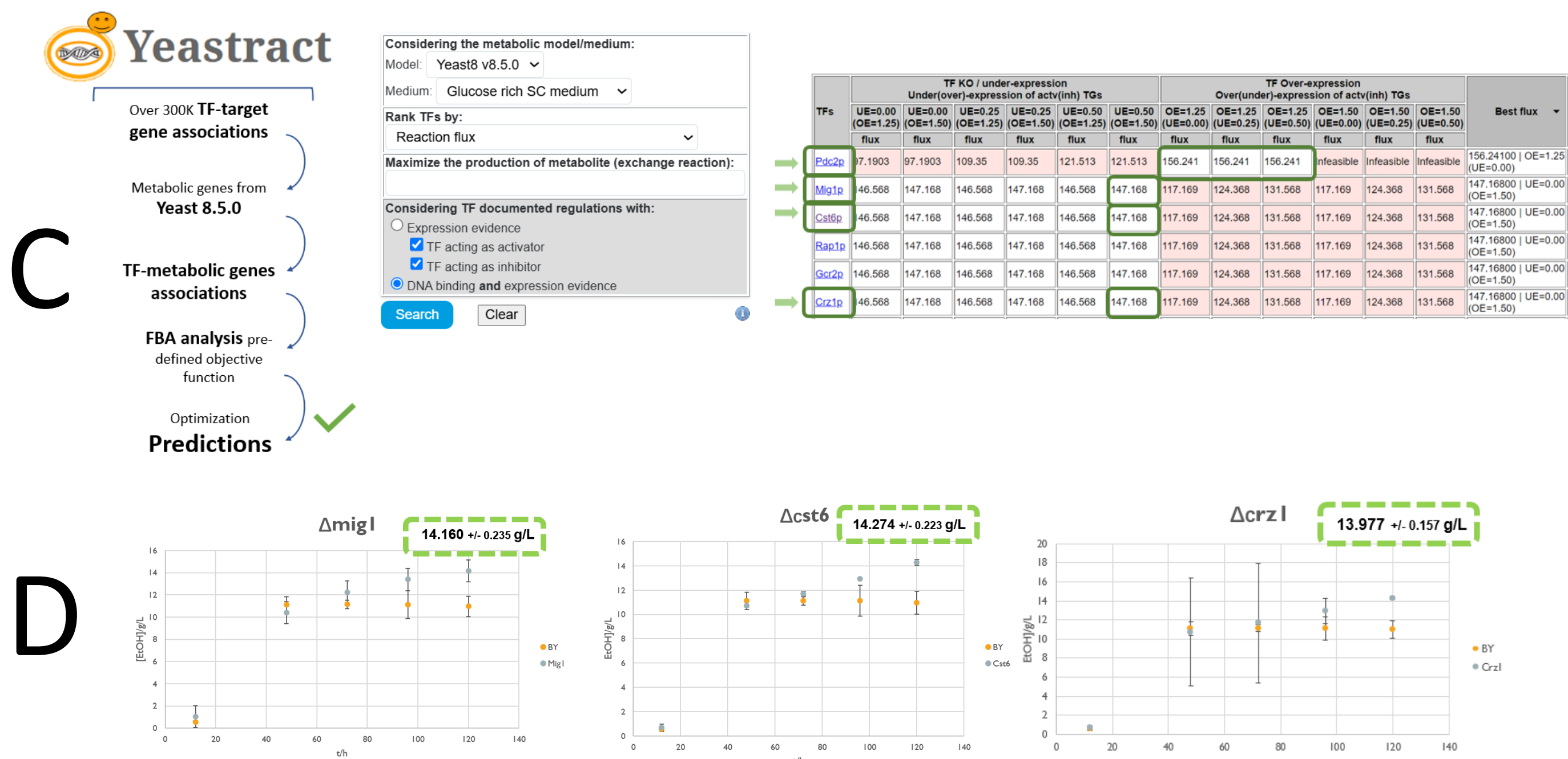
Figure: C) YeastRACT already allows for metabolite optimization by manipulating TF expression, with integration of 160 TFs. D) Wet-lab quantification validates in silico predictions for the three best single deletion mutants for the TFs MIG1p, CST6p and CRZ1p, all producing more ethanol than the around 11g/L produced by the wt. A 30% increase!
