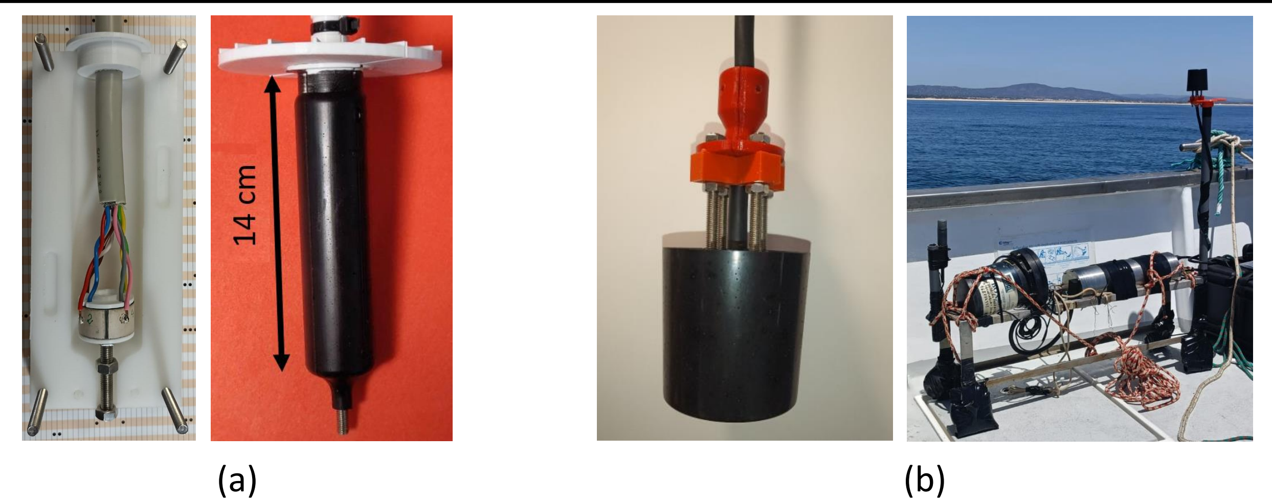
Figure 3: Developed Spiral Source Prototypes: (a) high frequency prototype before and after potting, and (b) low frequency prototype and the secondary devices for sea operation.
