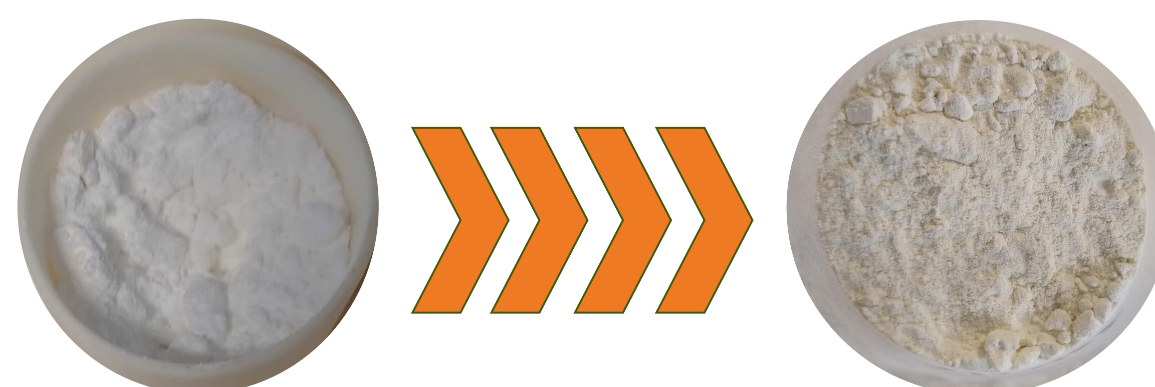
Figure 3 Representative pictures of yttrium and europium oxalate decahydrate (at the left) and yttrium and europium oxides (at the right).
