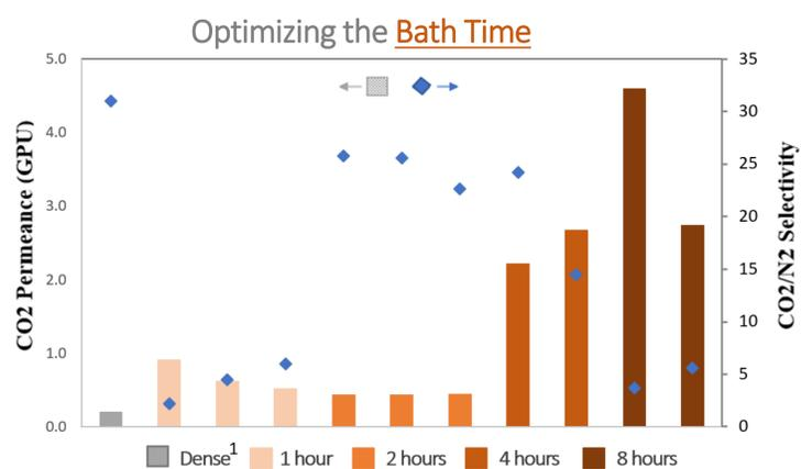
The CO<sub>2</sub> and N<sub>2</sub> permeances measured at T=20 °C of some of the prepared membranes are displayed below, as well as those of the dense PIL-20 IL NTf<sub>2</sub> membrane for comparison. Two different variables were studied, evaporation time and bath time.
