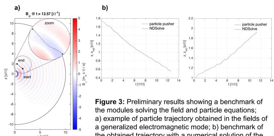
**Figure 3:** Preliminary results showing a benchmark of the modules solving the field and particle equations; a) example of particle trajectory obtained in the fields of a generalized electromagnetic mode; b) benchmark of the obtained trajectory with a numerical solution of the equations of motion (NDSolve).
