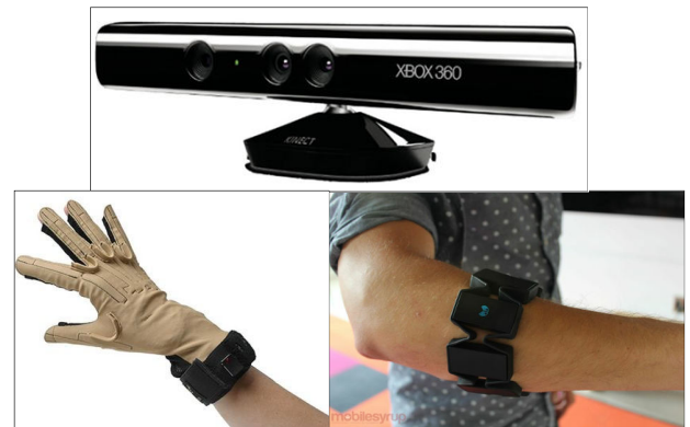
Figure 2. Sensors for the movement data acquisition: Kinect device (top), data glove (bottom left) and Myo sensor (bottom right)
